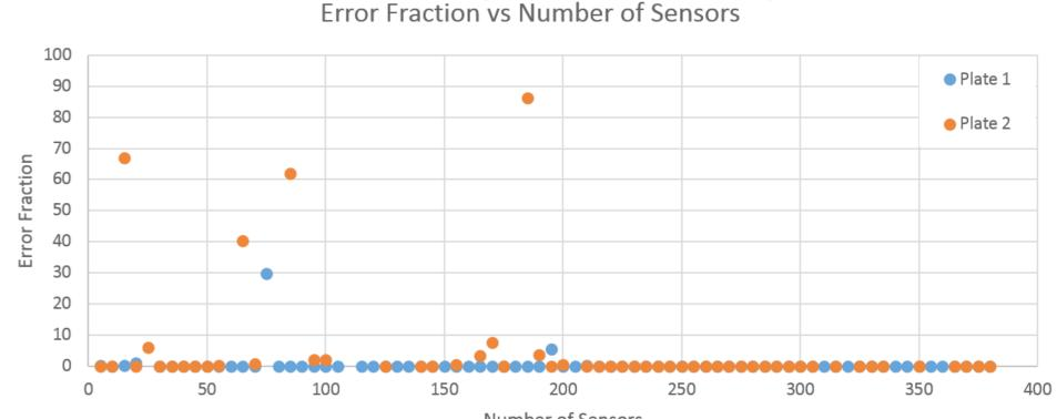
Number of Sensors Two things stand out: sometimes, with no apparent pattern, a highly inaccurate result is obtained. Second, even with quite a small number of sensors, an accurate estimate of the displacements can be obtained for a simple load case and a simple structure.
