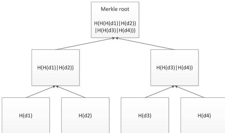
**Fig. 2** Example of a Merkle tree for four data elements
