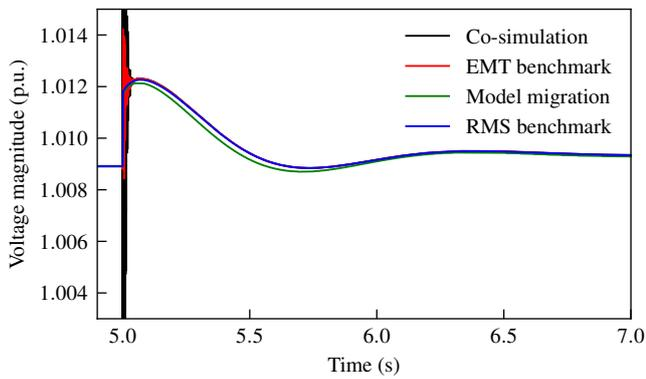
Fig. 7. Voltage magnitude at load  $L_2$  ( $V_L$ ) during a total loss of load  $L_1$ .
