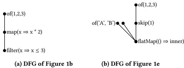
**Figure 2: Simplified DFGs corresponding to examples in Figure 1**
