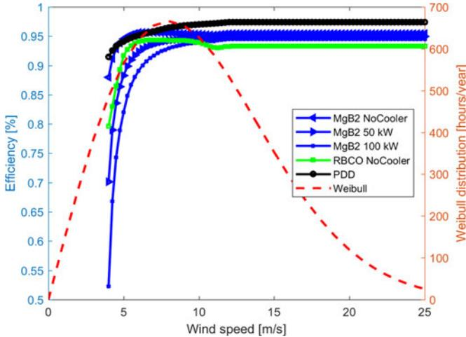
Fig. 4. Efficiency of the 10 MW MgB<sub>2</sub> generator with a constant power consumption of the cryogenic cooling system of 0, 50 kW and 100 kW [11], a 10 MW coated conductor RBCO based generator [3] without cryogenic cooling consumption and the magnetic Pseudo Direct Drive (PDD) generator [4] investigated in the INNWIND.EU project [16]. The Weibull wind distribution is shown on the right hand axis.
