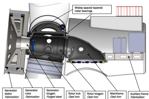
Fig. 1. Cross section view of the INNWIND.EU nacelle with the 10 MW MgB<sub>2</sub> generator mounted in front of the turbine blades [12]. The inner and stationary structure of the generator is attached to the stationary kingpin going through the rotor hub and connected to the main frame.
