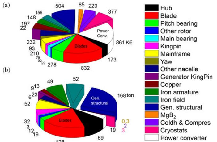
Fig. 3. 10 MW  $MgB_2$  superconducting direct drive wind turbine rotor, generator and nacelles component cost and weight breakdown [11]. a) Component cost in [k€] and b) component weight in [ton] according to the components outlined in [12]. The components associated with the superconducting drive train have been displaced from the center.
