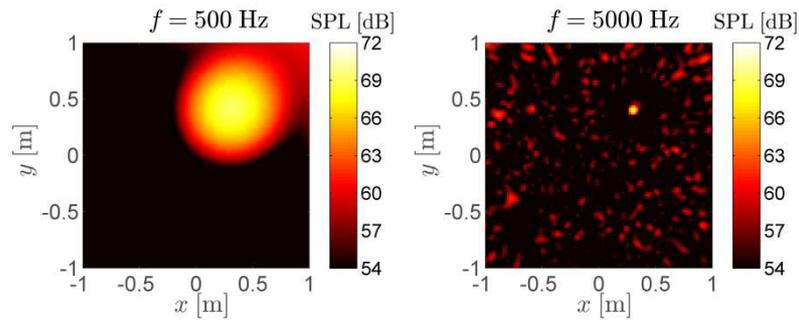
Figure 2: Beamforming for 500 and 5000 Hz.
