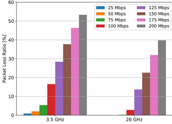
Figure 8: PLR for different required application bit rates.
