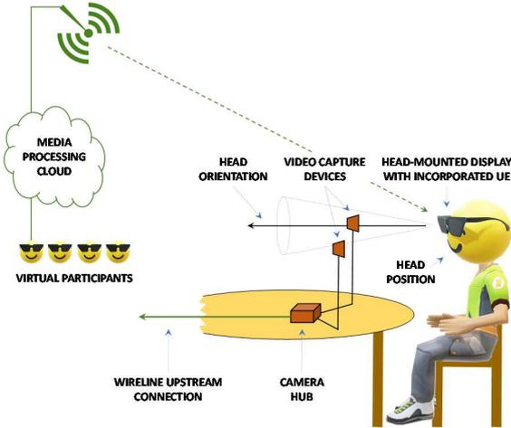
Figure 2: Illustration of user setting and end-to-end architecture.
