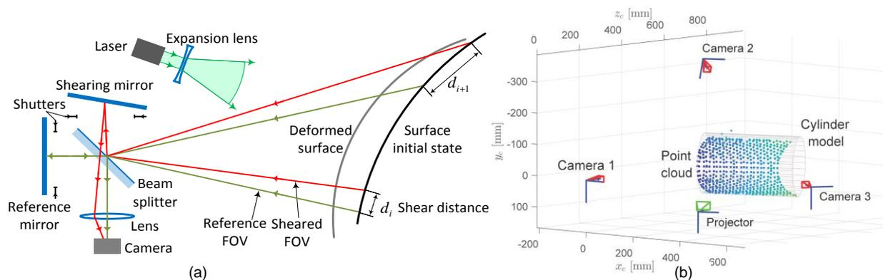
Fig. 1. 3D shape shearography: (a) schematic representation of the shearing camera and the shearing device based on a Michelson interferometer, (b) result of cameras-projector geometry calibration together with a point cloud corresponding to a cylinder specimen and a fitted cylinder model.
