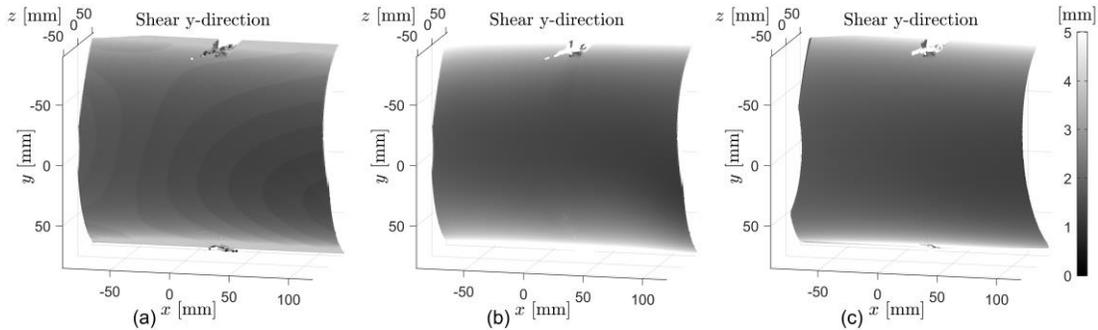
Figure 3. Shear distances in 3D estimated for camera 1 in the  $y$ -direction: (a) by searching the "nearest point of the point cloud", (b) by intersection with a fitted cylinder model and (c) by triangulation of the intersection within each facet.
