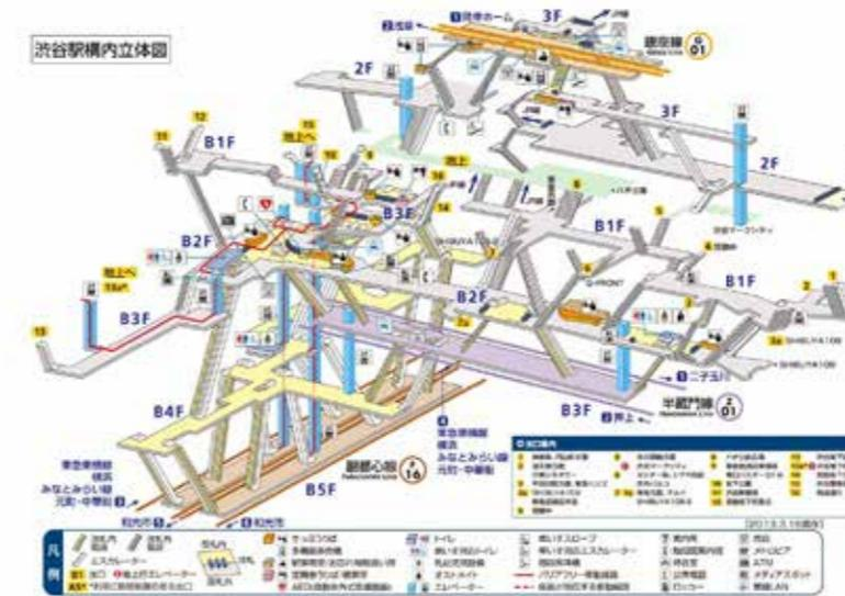
Fig. 11 The multiple tunnels and staircases connecting the various railroads crossing each other in Shibuya ([http://cdn.deepjapan.org/content/images/user/\\_image2\\_1\\_iM\\_OAg1396409208484.jpg](http://cdn.deepjapan.org/content/images/user/_image2_1_iM_OAg1396409208484.jpg)).
