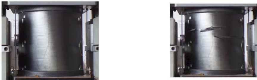
Figure 11. Photos of shell without cut-outs taken immediately before and after the collapse.
