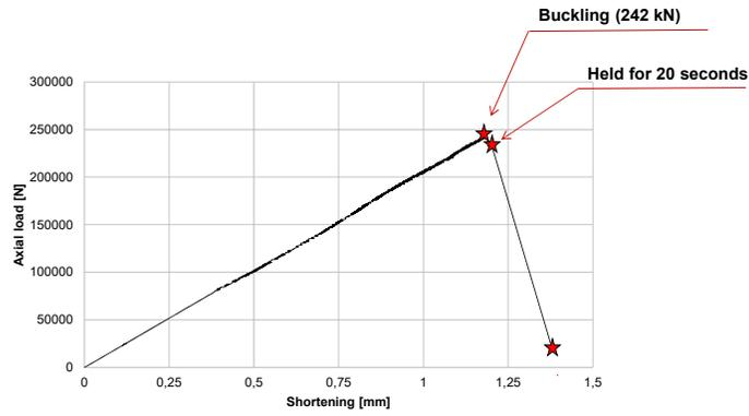
Figure 9. Load-shortening curve of shell without cut-outs.
