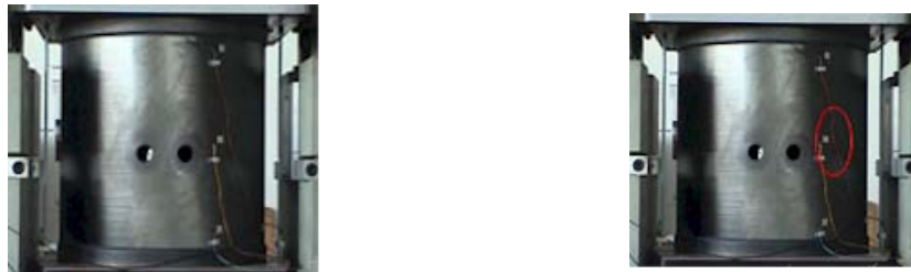
Figure 13. Photos of shell with cut-outs taken before and after buckling on the front side.
