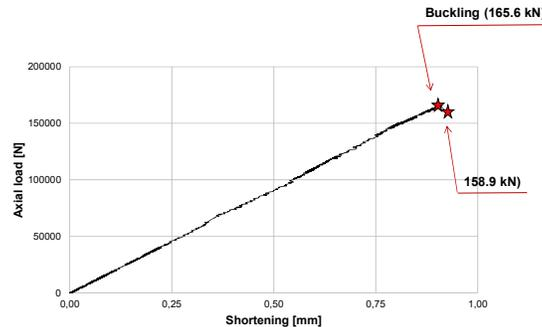
Figure 12. Load-shortening curve of shell with cut-outs.
