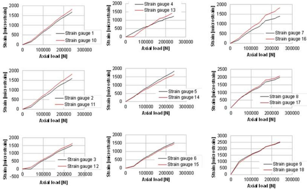
Figure 10. Strain gauges measurements of shell without cut-outs.
