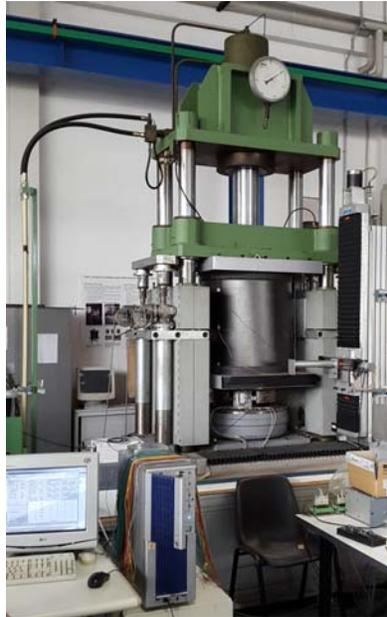
Figure 8. Buckling testing equipment.
