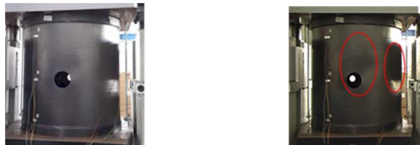
Figure 14. Photos of shell with cut-outs taken before and after buckling on the back side.
