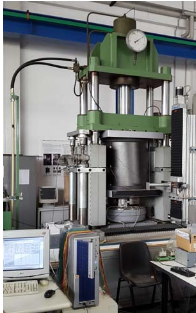
Figure 8. Buckling testing equipment.
