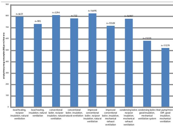
Figure 3 Primary energy consumption [MJ] per building cluster
