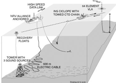
Figure 1: Overview of the measurement configuration. The data are acquired on a 64 hydrophone vertical line array (VLA). A sound source was mounted on a tower placed on the bottom. A ship (INS Ciclope) was measuring the sound speeds in the water column with conductivity-temperature-depth (CTD) sensors.
