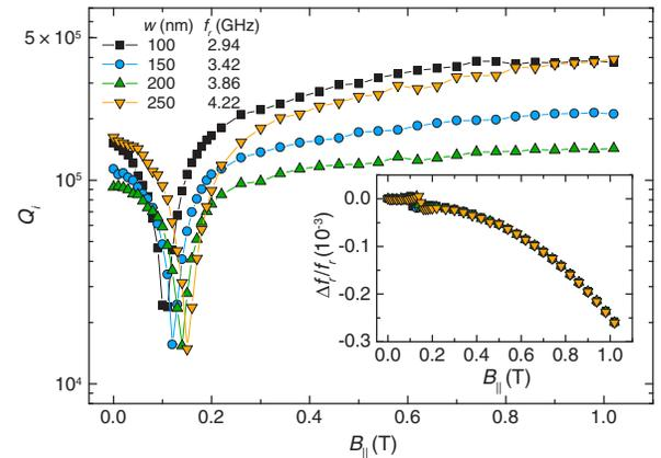
FIG. 7.  $B_{\parallel}$  evolution of  $Q_i$  in the four narrowest nanowire resonators shown on Fig. 4. (Inset) Fractional shifts of the four resonance frequencies as a function of the applied field. Symbols correspond to those in the main figure.
