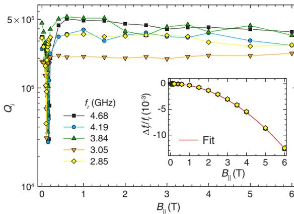
FIG. 3. Evolution of nanowire resonator characteristics with an in-plane magnetic field  $B_{\parallel}$  ( $w = 100$  nm,  $T = 280$  mK,  $P_{\text{in}} \approx -110$  dBm). The intrinsic quality factor  $Q_i$  remains unaffected in the range  $400 \text{ mT} \lesssim B_{\parallel} \leq 6$  T. The maximum  $B_{\parallel}$  is limited by our experimental setup. (Inset) All fractional frequency shifts fit to the same simple quadratic curve.
