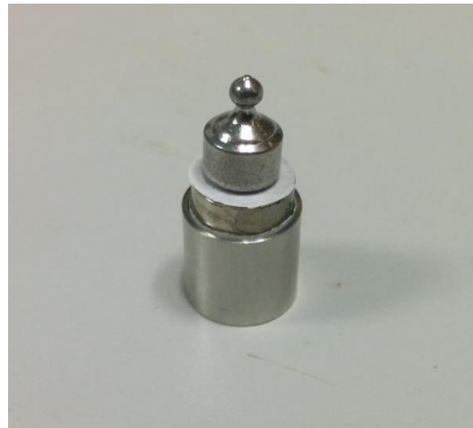
3 FIGURE 4 a. Sample in Storage Container, Showing the Silicon Paper That Controls Contact Area d. 4 Assembled Test Specimen with Weight.
