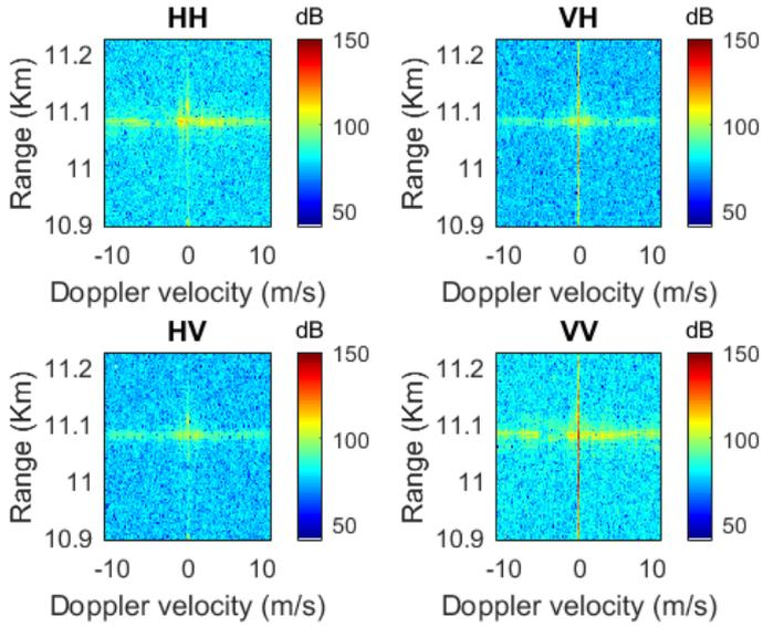
Fig. 4. Range-Doppler spectrogram of wind turbine clutter.
