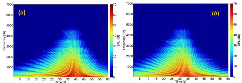
Figure 3: Audio spectrograms of an A320 approaching an airport – (a) Reference aircraft, (b) Low tonality aircraft variant [5]
