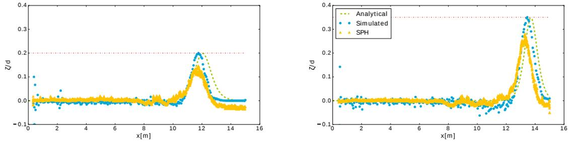
Fig. 5. Comparison between the analytical, the hybrid particle-mesh and the SPH solution for the generated solitary wave at  $t = 8$  s. The left panel corresponds to the  $H/d = 0.2$  case, the right panel corresponds to the  $H/d = 0.35$  case.
