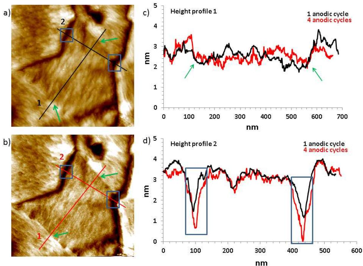
Fig. 4 Topographic ECSTM images of metallic surface of polycrystalline copper after (a) 1 and (b) 4 anodic cycles ( $X = Y = 700 \text{ nm}$ ,  $\Delta Z = 4 \text{ nm}$ ,  $E_{\text{Cu}} = -0.05 \text{ V}$ ,  $E_{\text{tip}} = -0.35 \text{ V}$ ,  $I_{\text{tip}} = 2 \text{ nA}$ ) and height profiles along (c) line 1: Green arrows mark coherent twin grain boundaries and (d) line 2: blue rectangles mark random grain boundaries [3].
