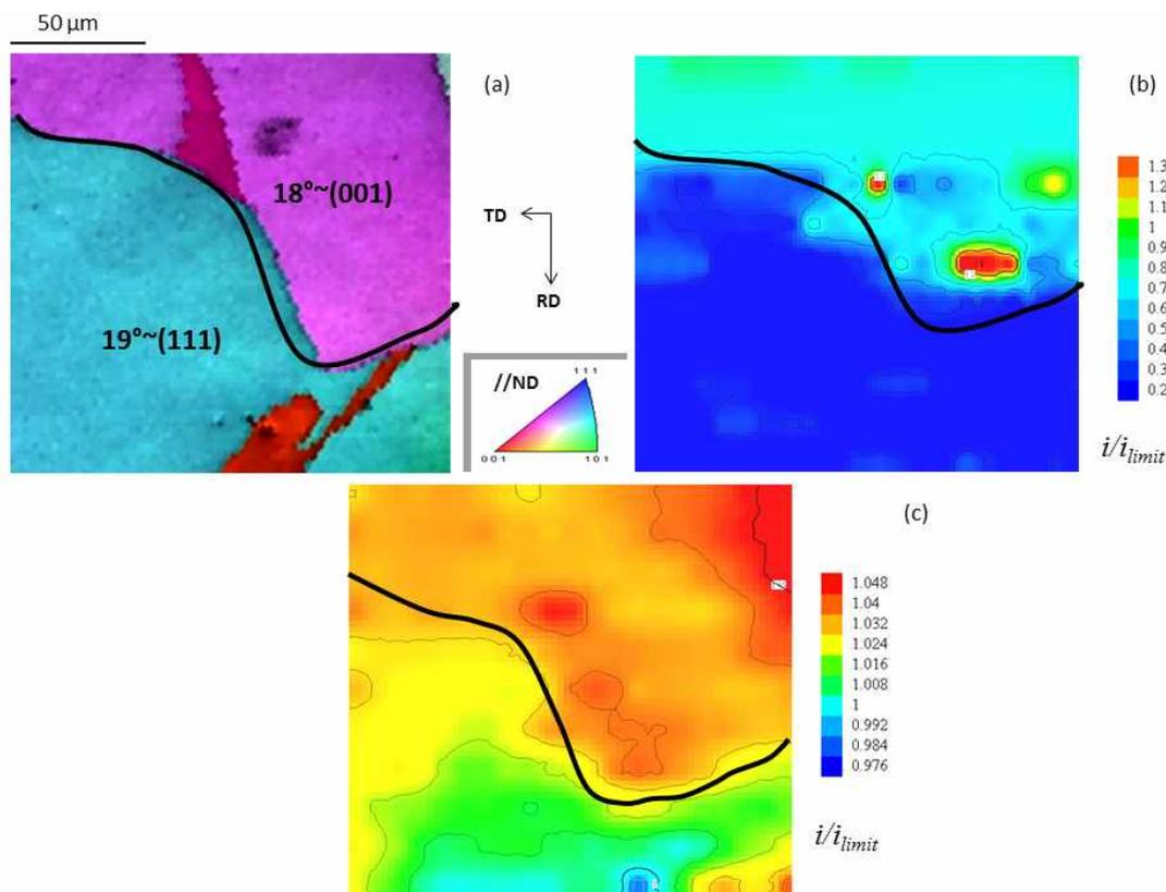
**Fig. 3** Combined inverse pole figure (IPF)/image quality (IQ) map (a) and corresponding SECM current map after passivation at  $E = 0.1$  V during 30min (b) corresponding SECM current map after the cathodic reduction of the passive layer (c). Measurements in sodium hydrogen orthophosphate/sodium hydroxide buffer solution containing 5mM ferrocenemethanol. Scanned area  $200 \mu\text{m}$  in x and y direction with  $dx=10 \mu\text{m}$  and  $dy=20 \mu\text{m}$  [2].
