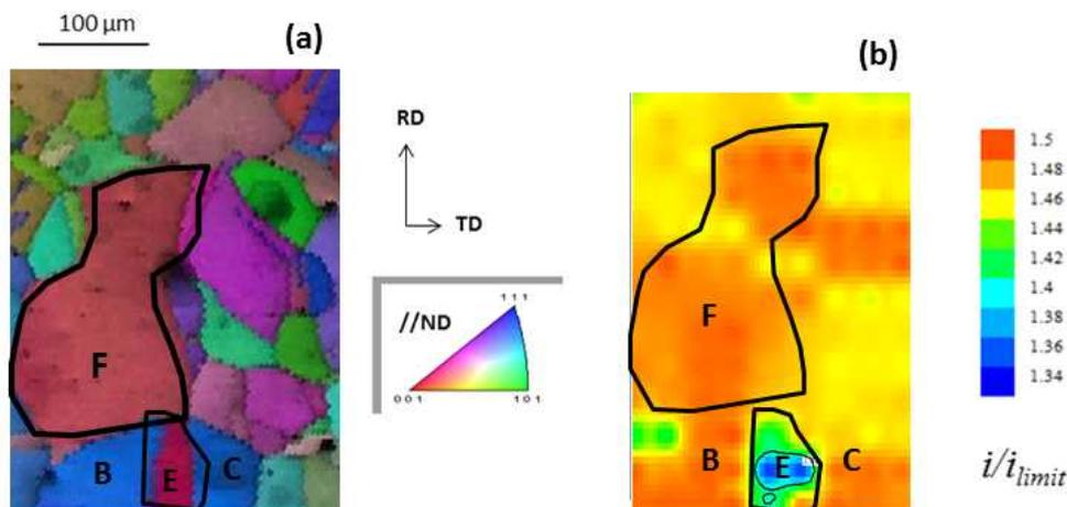
**Fig. 2** Combined inverse pole figure (IPF)/image quality (IQ)map (a) and corresponding SECM current map (b). Scanned area  $400\mu\text{m}$  in x and y direction with  $dx=10\mu\text{m}$  and  $dy=20\mu\text{m}$ , experiments in the active dissolution state. Area involving  $\langle 111 \rangle // \text{ND}$  (B and C) and  $\langle 001 \rangle // \text{ND}$  (E and F) oriented grains [2].
