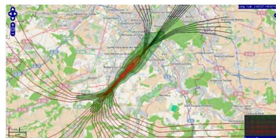
Figure 6: Noise contours associated to different trajectories, STAPES.
