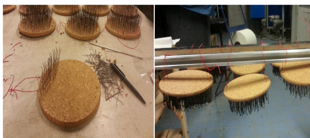
Figure 1: Bitumen coating of steel fibres.
