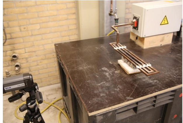
Figure 3: Set-up of induction heating and infrared camera measurements.
