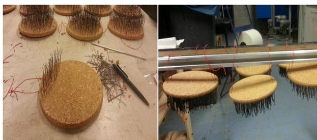
Figure 1: Bitumen coating of steel fibres.
