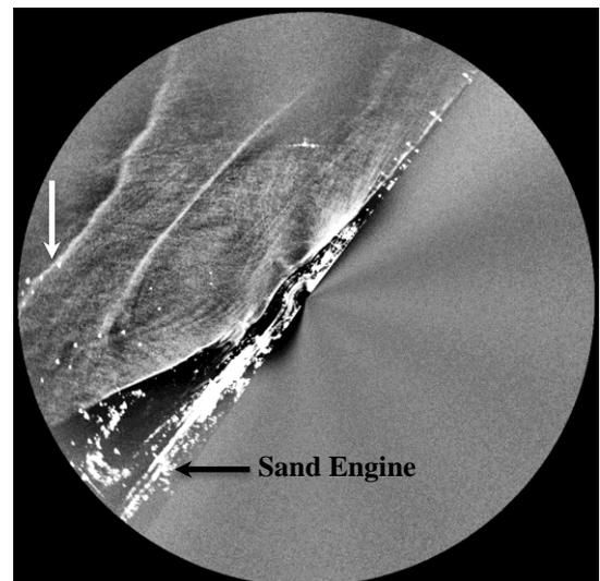
Figure 2. X-band radar image of the 1<sup>st</sup> of October 2014 at 19:10:00 UTC. The upper white dots are buoys and the measurements at 12m depth. At this moment a front passes through the measurement site.
