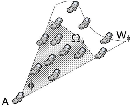
Fig. 5. Demonstration of the directional PLE estimation in  $\mathbb{R}^2$ .  $A$  is the considered node collecting the RSSs from within the angle  $\phi$ .  $W_\phi$  is the actual transmission range bounded by  $\phi$ , and the shaded area  $\Omega_\phi$  is the corresponding sector with radius  $r$ .
