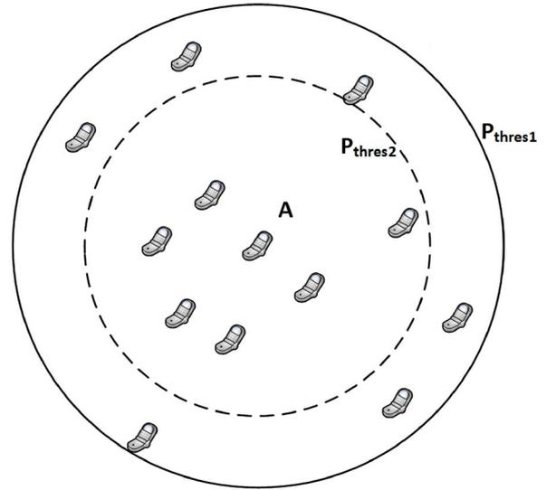
Fig. 6. Demonstration of the C-PLE estimator. Node  $A$  changes its receiver's sensitivity from  $P_{thres1}$  to  $P_{thres2}$ . The solid circle and the dashed circle are, respectively, the transmission ranges related to  $P_{thres1}$  and  $P_{thres2}$ . The corresponding neighborhood sizes are  $\hat{n}_1 = 12$  and  $\hat{n}_2 = 6$  in this figure. The estimated PLE can be obtained from (35).
