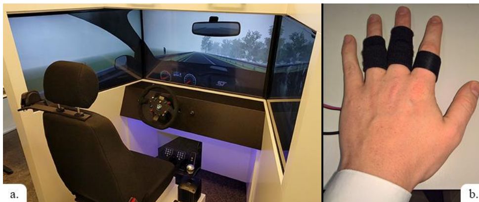
Figure 1: (a) The GreenDino fixed-base, medium-fidelity driving simulator; (b) Demonstration of physiological sensors attached to the left hand. The PPG sensor is placed at the index finger, the GSR sensor cuffs at the middle and ring finger.
