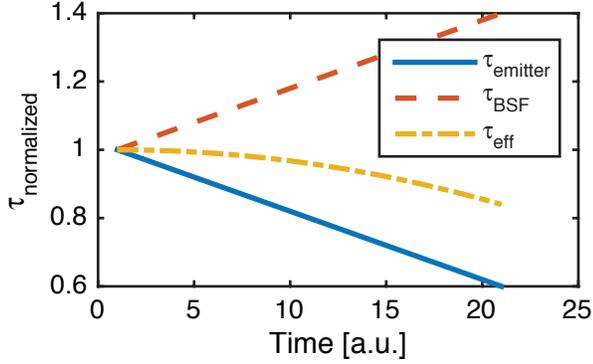
Fig. 10. Calculation of  $\tau_{\text{eff}}$  under the assumption that  $\tau_{\text{emitter}}$  and  $\tau_{\text{BSF}}$  change according to the curves given in Figure 6. Simulated  $\tau_{\text{emitter}}$  and  $\tau_{\text{BSF}}$  is also shown here.  $\tau_{\text{bulk}}$  is ignored so  $\tau_{\text{eff}} = \left( \frac{1}{\tau_{\text{emitter}}} + \frac{1}{\tau_{\text{BSF}}} \right)^{-1}$
