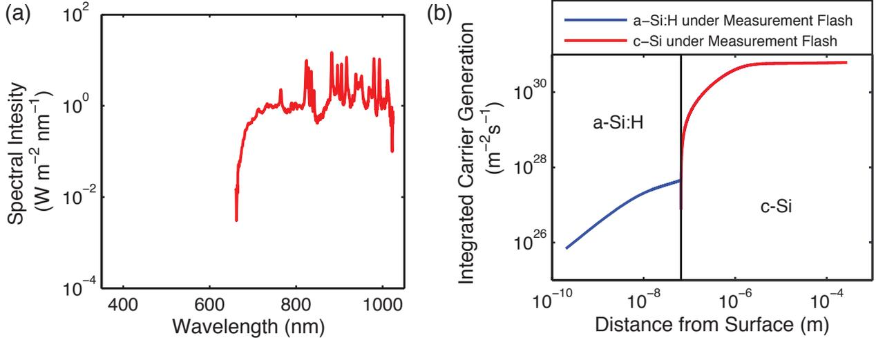
Fig. 1. (a) Light spectrum of flash of Sinton PCD lifetime tester. (b) Cumulative generation profile of samples. The generation profile has been integrated to show how many charge carriers per  $\text{cm}^2$  are generated in the a-Si:H film and the c-Si wafer.
