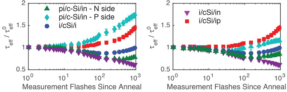
Fig. 6. MEPCD measurement on precursor stack as well as other stacks shown in Figure 5. The two figures presented here obtain the same measurements for the *i/i* and single doped layer samples. However in the case of the precursor sample, in (a) the emitter side was illuminated first, while in (b) the back surface field side was illuminated first.
