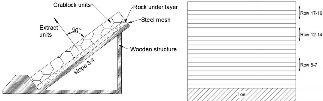
Figure 5: Test set up of pull tests
