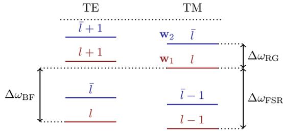
FIG. 3. Spectrum of WGMs: the resonant frequency of a WGM depends on the angular momentum ( $l_R$ ), the number of radial nodes ( $\nu - 1$ ), and the polarization. This sketch includes the levels for the first two radial modes  $\nu = 1$  and 2 denoted by red and blue, respectively. The labels FSR, BF, and RG are defined in the text.
