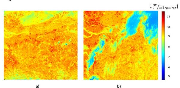
Fig. 3. Synthetic high resolution TIR image (a) and existing TIR Landsat-8 (b) in radiance values from the same date.
