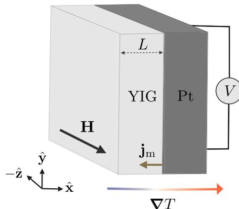
FIG. 1. Pt|YIG bilayer subject to a thermal gradient  $\nabla T \parallel \hat{\mathbf{x}}$  and a magnetic field  $\mathbf{H} \parallel \hat{\mathbf{z}}$ . The thermal bias gives rise to a flow of magnons, i.e., a magnonic spin current  $\mathbf{j}_m$ , in the YIG film of thickness  $L$ . In the Pt lead, the spin current is then converted into a measurable voltage  $V$  via the inverse spin Hall effect.
