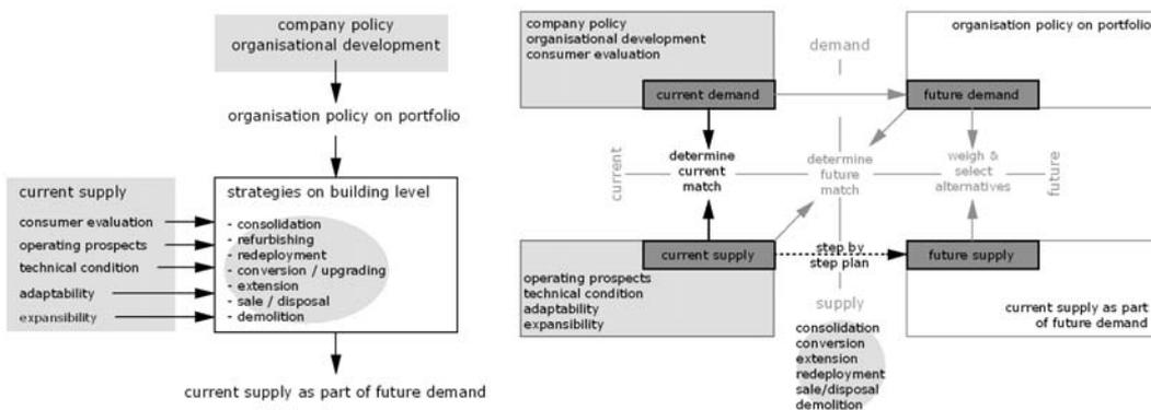
Fig. 7. Accommodation assessment (left), combined with the DAS-Framework (right)
