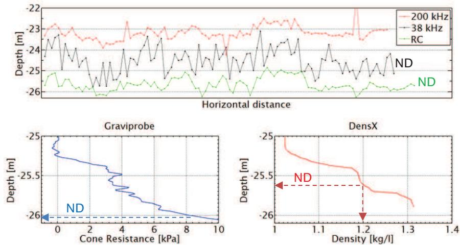
Fig. 1. Characterization of the fluid mud layer by means of the echo-sounder, Rheocable, Graviprobe and DensX. 'ND' stands for the nautical depth.
