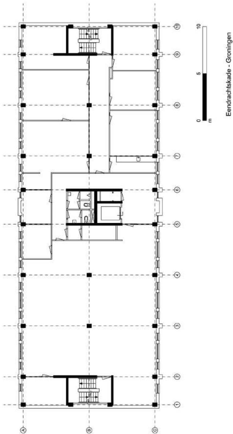
Figure 2. Typical floor plan before conversion of the office building into housing.
