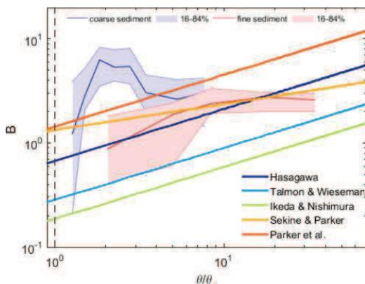
Figure 2. Range in slope factor of the experiments with fine and coarse sediments, compared with existing predictors that include a ratio of sediment mobility ( $\theta$ ) to critical sediment mobility ( $\theta_c$ ).
