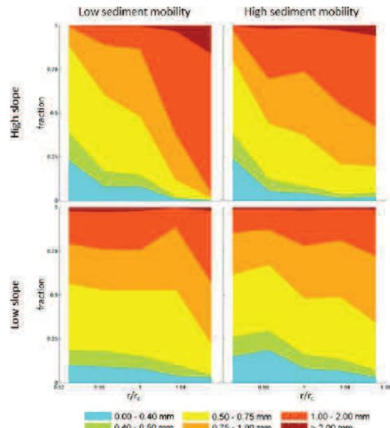
Figure 3. Fraction of grain sizes at several locations along the cross-section relative to flume radius ( $r/r_c$ ), for experiments with high and low transverse slopes, and high and low sediment mobility.
