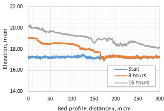
Figure 14. Bed topography profile after 0, 8, and 16 hours.
