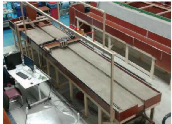
Figure 13. Sand-bed flume, with sediment feeder in the upstream and laser recorders.
