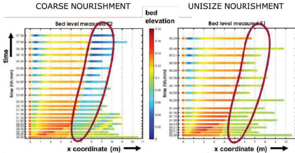
Figure 1: Laboratory experiment with nourished sediment located at  $x = 0$  and  $x = 3.5$  m at time 0 for two cases (nourished sediment coarser than bed surface sediment (left) and unisize compared to bed surface sediment (right)). In a case of coarse nourishment degradational wave is migrating downstream considerably faster than the nourished sediment. (from Blom 2016)
