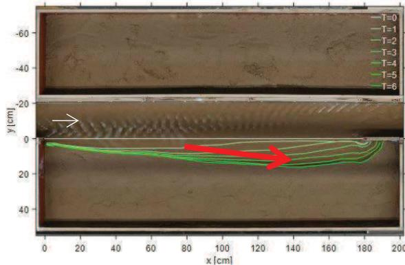
Figure 1. Evolution of bank line with time  $T$  in hours in experimental test with bank protection removal length of nine times the channel width on one side of the channel. Red arrow indicates channel widening in downstream direction.
