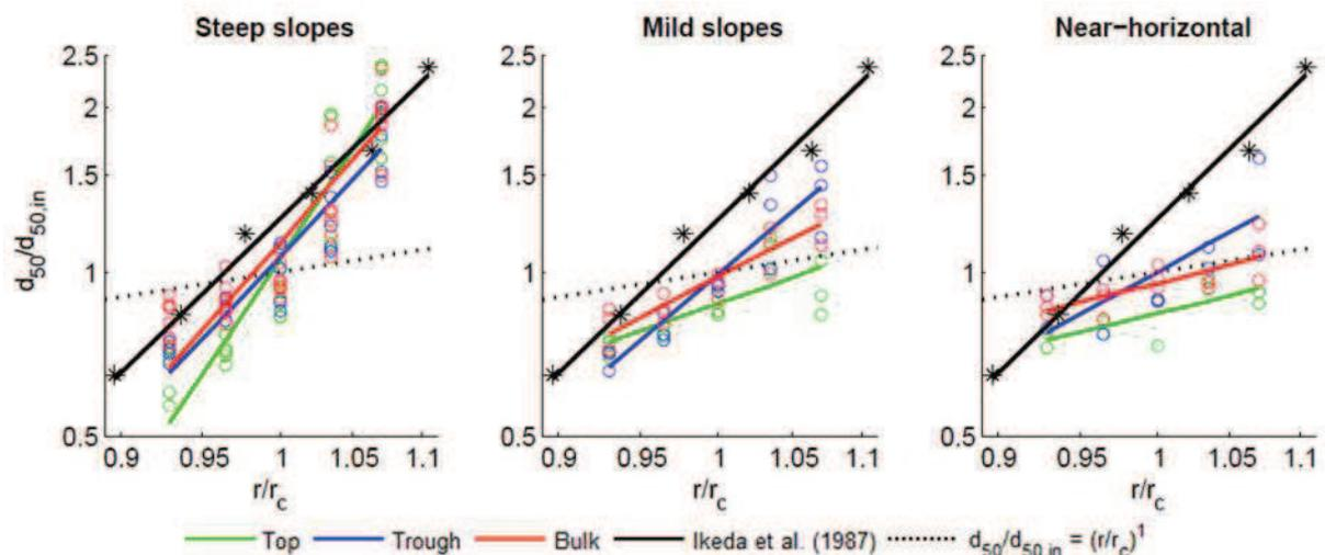
Figure 26. Relative median grain size over the width of the flume.  $d_{50,in}$  = median grain size of initial, unsorted mixture,  $r$  = local radius and  $r_c$  = radius at channel axis. Power of power fit increases with transverse slope, indicating a larger transition from fine to coarse.
