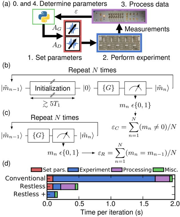
FIG. 1. (a) A general qubit-gate-tuneup loop. In conventional tuneup (b), the qubit is initialized before measuring the effect of  $\{G\}$ . In restless tuneup (c), the qubit is not initialized, and instead  $m_{n-1}$  is used to estimate the initial state ( $|\tilde{m}_{n-1}\rangle$ ). (d) Benchmark of various contributions to the time per iteration in conventional and restless tuneup, without and with technical improvements (see text for details).
