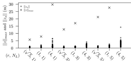
Figure 5: Plot of the simulation ( $\|z_s\|$ ) and the theoretic ( $\|z\|_{max}$ ) bounds, for different combinations of the  $r$  and  $N_L$  parameters. The  $\|z\|_{max}$  values for  $(r, N_L) = (1, 3)$  and  $(4, 5)$  are out of scale and are not shown for the sake of clarity.
