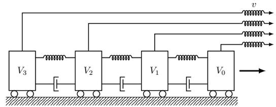
Figure 3: Spring-damper representation of the proposed control system.
