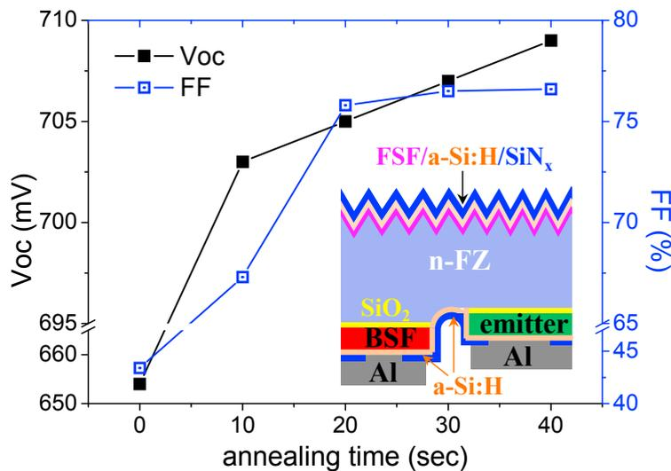
Fig. 5. The  $V_{OC}$  and FF of IBC solar cells with FSF passivated with a-Si:H/SiN<sub>x</sub> as a function of annealing time at 600 °C. Inset picture depicts cross sectional sketch of half pitch of IBC cell #5 and #6. The annealing is done step by step, with 10-second long steps.
