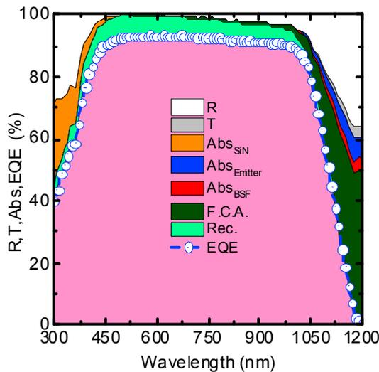
Fig. 3. The measured external quantum efficiency (EQE) of cell #4 (see Table 2), the reflectance (R) and transmittance (T) which are plotted as 1-R-T. The loss analysis is conducted by accurate TCAD Sentaurus optical-electrical simulator [10].
