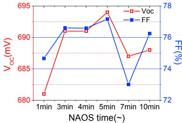
Fig. 2. V<sub>oc</sub> and FF of fabricated IBC cells plotted against the single step NAOS-SiO<sub>2</sub> immersion time (69% HNO<sub>3</sub> bath at 110 °C).
