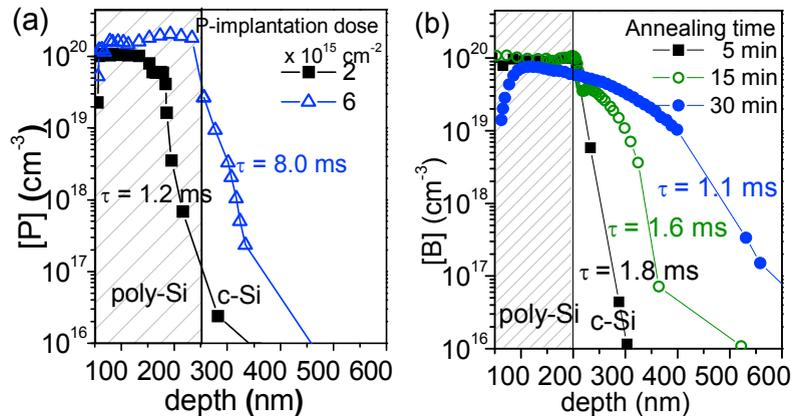
Fig. 1. (a) P-doping profile of 250-nm thick poly-Si passivating contacts (20 keV implantation energy and annealing at 950 °C for 5 min in N<sub>2</sub>, but different implantation dose). (b) B-doping profile for 200-nm thick poly-Si passivating contacts (5 keV implantation energy, implantation dose of  $5 \times 10^{15} \text{ cm}^{-2}$  and annealing at 950 °C in N<sub>2</sub> but different annealing time).
