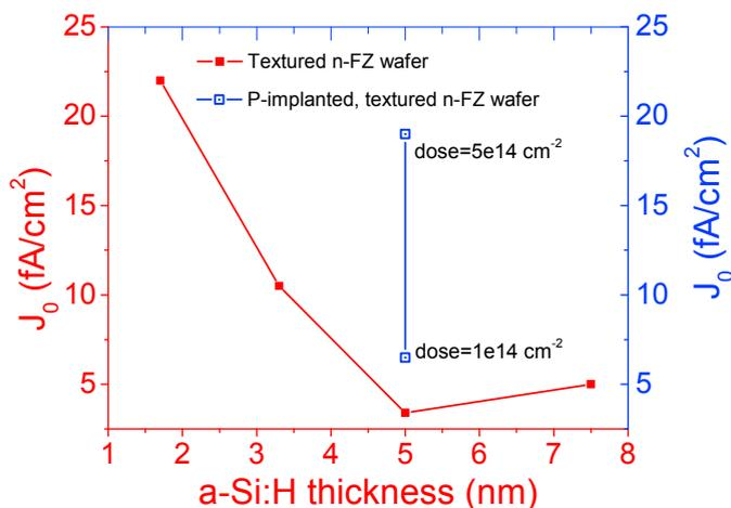
Fig. 4. Surface passivation quality ( $J_0$ ) of P-ion implanted textured n-FZ wafers, which can be deployed as front side of the IBC solar cells, coated by PECVD a-Si:H/SiN<sub>x</sub> stack as a function of the a-Si:H layer thickness and the doping level.
