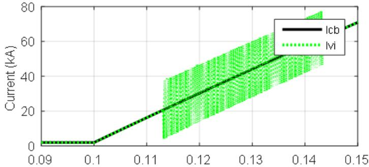
Figure 16 Current interruption with delayed trip signal
