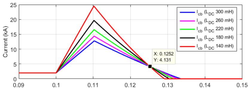
Figure 13 Comparison of  $I_{cb}$  with different  $L_{dc}$
