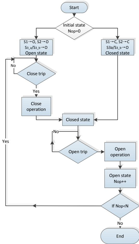
Figure 9 Flow chart of DC CB control sequence
