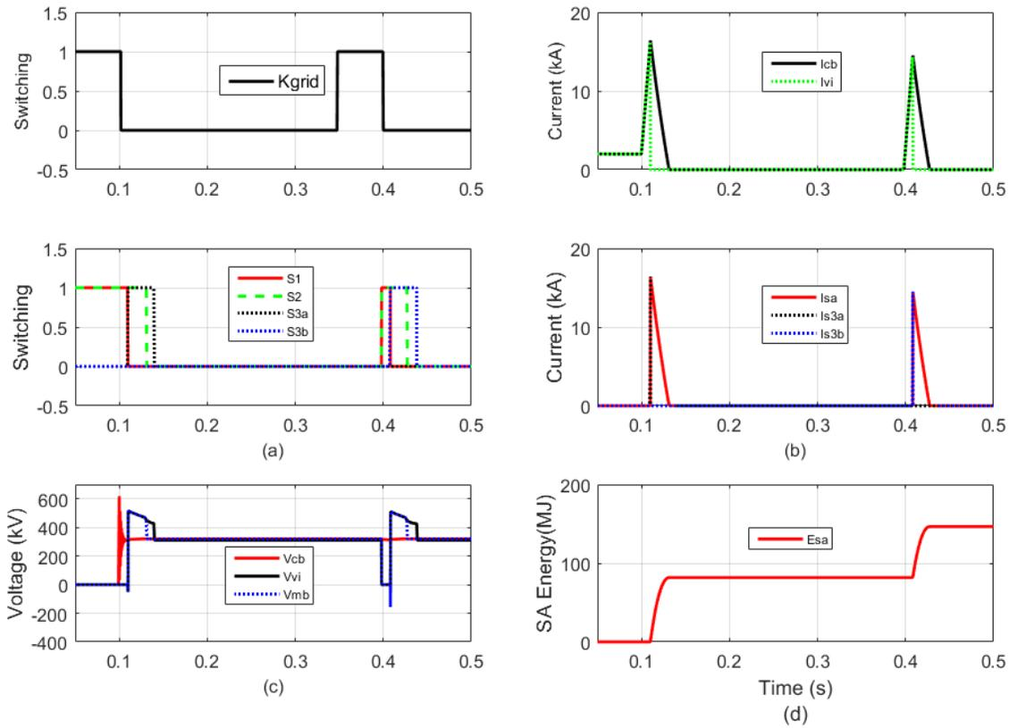
Figure 10 Repeated open-close cycle operation with dead time 250ms
