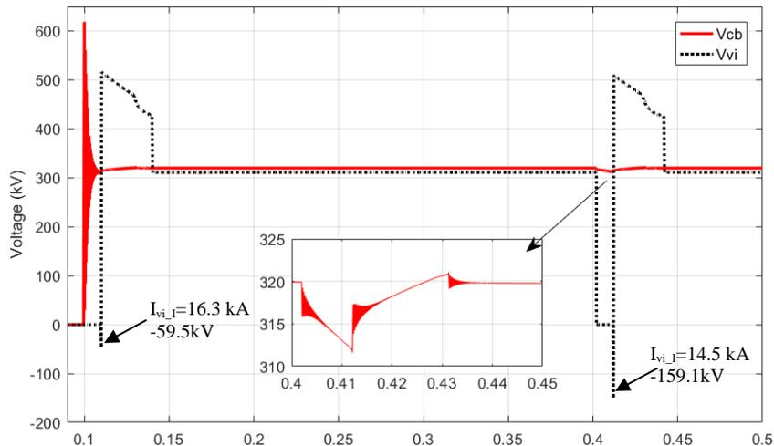
Figure 12  $V_{cb}$  variation during second close- open based on PSCAD
