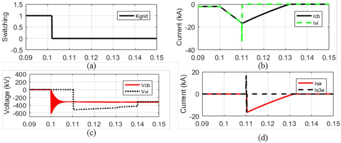
Figure 7 DC CB Reverse high current interruption performance on receiving grid order
