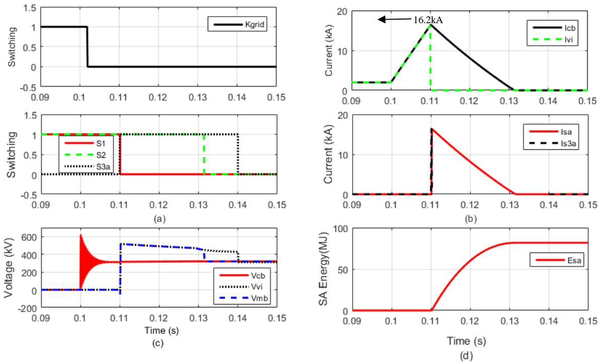
Figure 6 Rated Current Interruption on External Order (Mechanical DC CB) based on PSCAD
