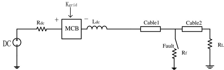
Figure 4 DC MCB verification circuit
