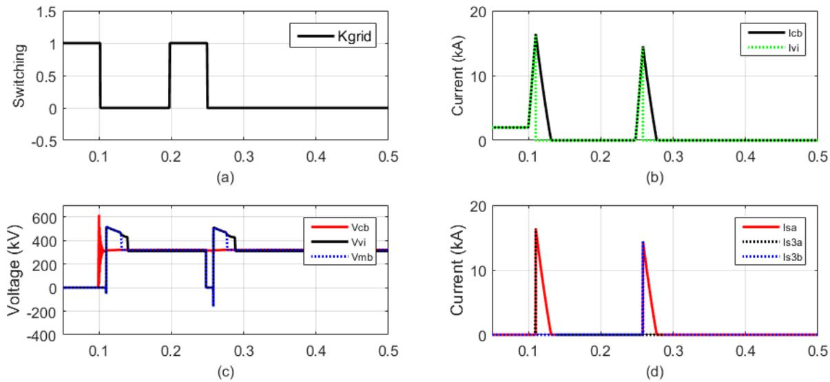
Figure 11 Repeated open-close cycle operation with dead time 100ms
