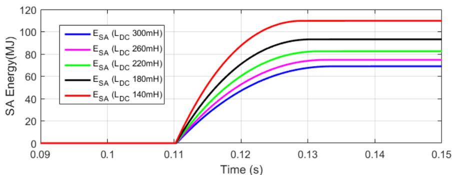
Figure 14 Comparison of  $E_{SA}$  with different  $L_{dc}$
