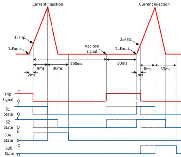
Figure 8 Sequence of repeat operation Mechanical DC CB
