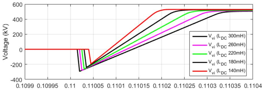
Figure 15 Comparison of TIV with different  $L_{dc}$
