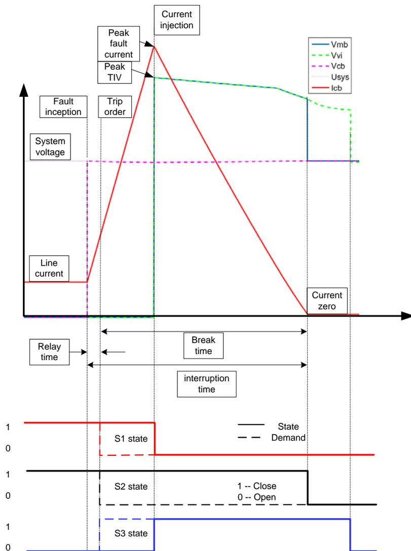
Figure 3 Relevant voltages and a circuit breaker current as well as associated switching states of the switches  $S_1$ ,  $S_2$  and  $S_3$  during fault current interruption.
