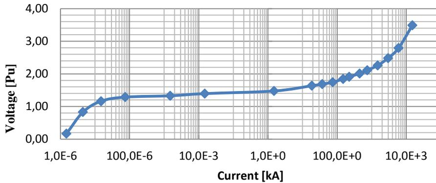
Figure 2 Aggregated surge arrester current-voltage characteristics
