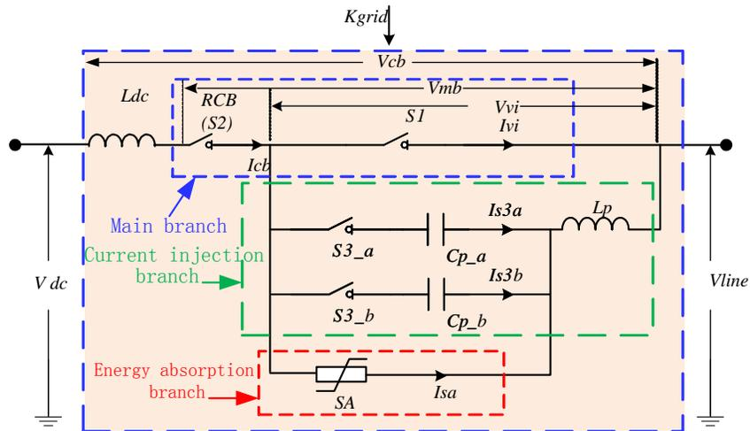
Figure 1 General topology of the mechanical DC CB with current injection
