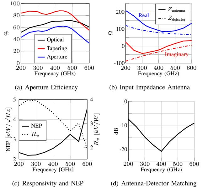
Fig. 3. Antenna’s aperture efficiency (a), Input impedance of both antenna and detector seen from terminals  $T1$  and  $T2$  in Fig. 1 (b), Simulated optimal NEP and responsivity including antenna-detector mismatch (c), Antenna-Detector mismatch at the terminals  $T1$  and  $T2$  in Fig. 1 (d).
