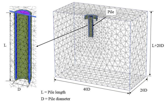
Figure 1. Typical mesh for three-dimensional finite element analyses
