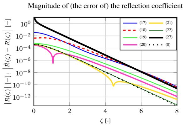
**Fig. 3:** Magnitude of (the error of) the reflection coefficient for a hyperbolic secant potential for the NSE. The numbers between brackets refer to the corresponding equation: (27): ground truth, (8): error without splitting (due to staircase approximation), (17)–(22): error with splitting.
