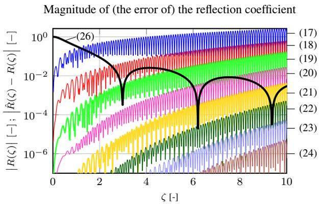
**Fig. 2:** Magnitude of (the error of) the reflection coefficient for a rectangular potential for the KdV. The numbers between brackets refer to the corresponding equation: (26): ground truth, (17)–(24): error due to splitting. The error without splitting (Eq. (8)) is zero here, because this potential equals its staircase approximation exactly.
