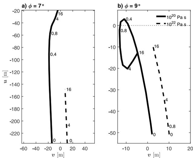
**Figure 4.** Horizontal and vertical displacement of the surface at (a) 7° and (b) 9° colatitude for both viscosities. For visibility, the curve for  $\eta = 10^{22}$  Pa s has been displaced horizontally by 25 m in (a) and 8 m in (b). Labels denote the time in kyr after removing the ice cap.
