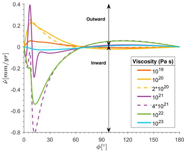
**Figure 1.** Present-day horizontal velocities ( $\hat{v}$ ) as a function of colatitude  $\phi$  for varying mantle viscosity as a result of the growth and melt of an axisymmetric ice cap with a radius of  $8^\circ$  (dashed vertical line) centered at the North Pole.
