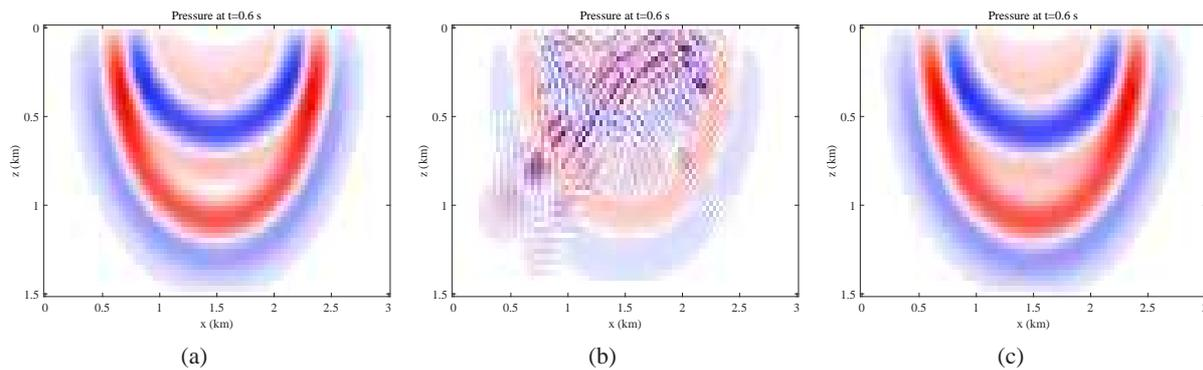
**Figure 2** Pressure field generated by a point source for (a) the second-order formulation with a delta-function point source, (b) the first-order formulation with a delta-function point source and no defect-correction iterations, and (c) with a gaussian source and two defect-correction iterations.
