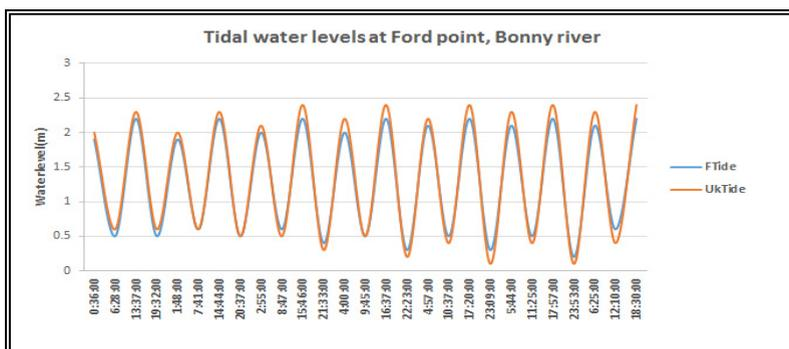
Fig.3. Comparison of two sources of tidal water level data for the Niger delta
