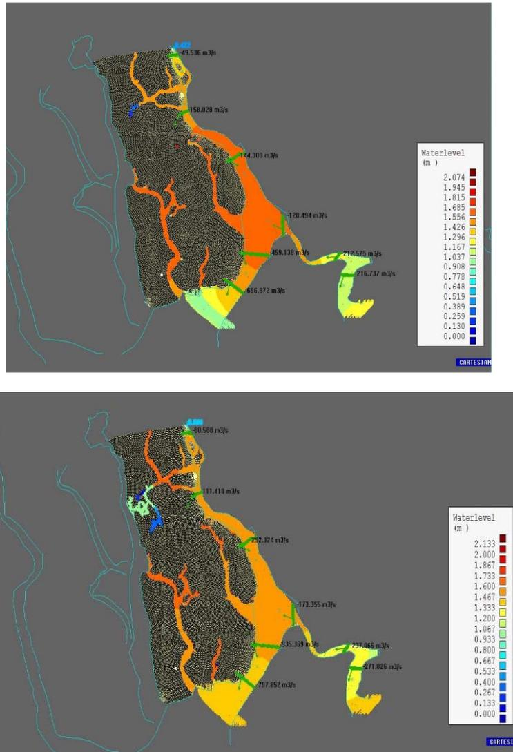
Fig.6: model results showing new areas covered by water with sea level rise. (Top) no SLR, (Bottom) SLR=0.4m.
