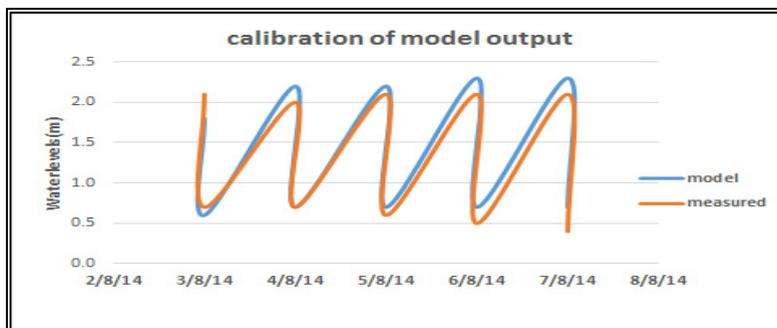
Fig. 4. Model calibration by comparing model result with tidal gauge data
