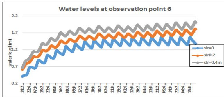
Fig. 5. Model water level output showing increase in water levels with sea level rise.
