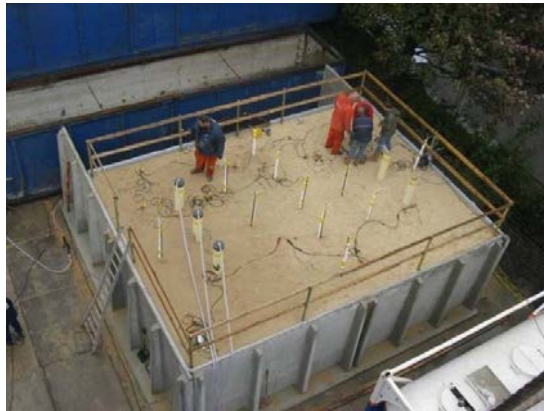
Figure 4. Pilot scale (100m 3 ) bio-grouting experiment by van Paassen and colleagues. Image courtesy of Leon van Paassen, Delft University of Technology
