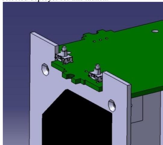
Figure 6 Deployment switches
