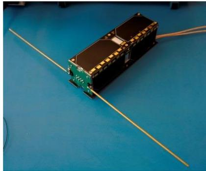
Figure 8 Deployed antennas
