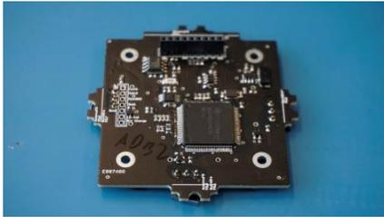
Figure 7 Antenna Board
