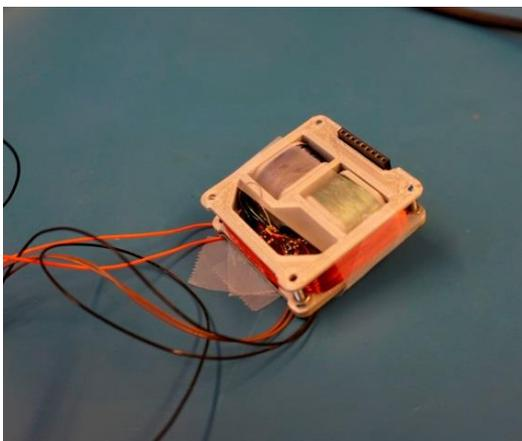
Figure 14 Magnetorquers
