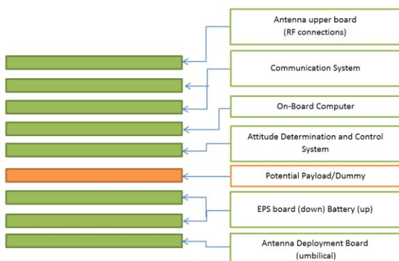
Figure 15 Satellite configuration
