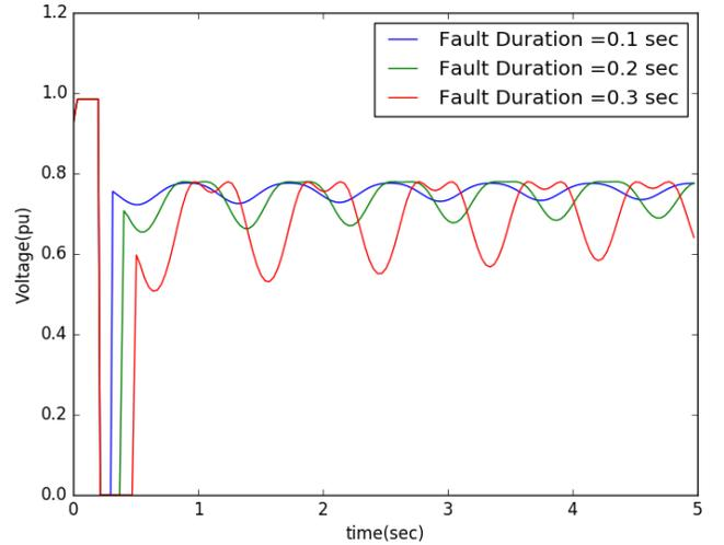
Fig. 8: Bus 5 voltage for FIDVR events with different fault durations.
