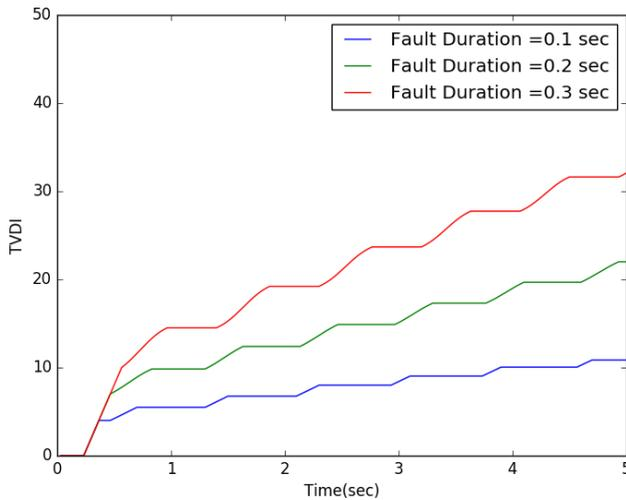
Fig. 9: TVDI calculation for FIDVR events with different fault durations.
