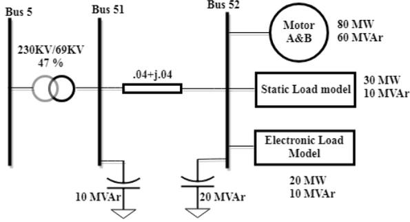
Fig. 4: Composite load model as specified in [20]
