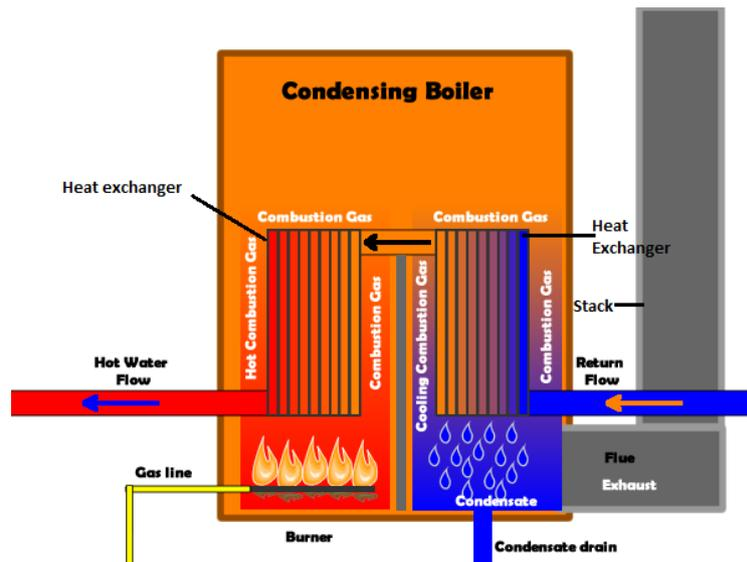
Figure 1. Condensing boiler.
